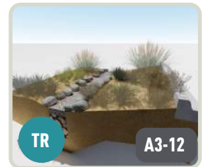
TR A3-12 INFILTRATION TRENCH
