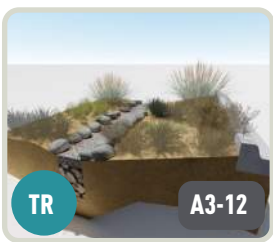
TR A3-12 INFILTRATION TRENCH
