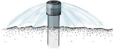
PVC and emitter components for typical bubbler irrigation systems
