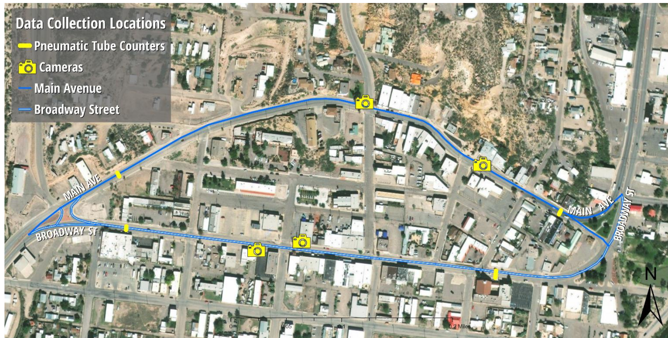
Figure 5: Video Camera and pneumatic tube deployments in Focus Area 1.
